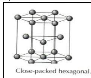
Fig. 2 Hexagonal close packed structure
