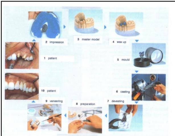
Fig. 5: Lost-wax casting method
