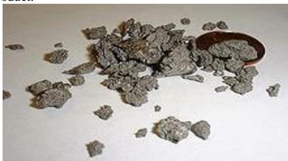
Fig. 1: Titanium sponge, made by the Kroll process
