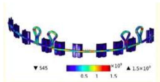
Figure 7: Frontal view showing Stress is concentrated in the loops.
