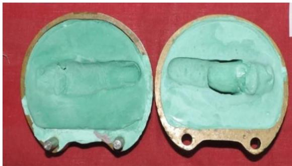
Figure 3: Moulds after dewaxing
