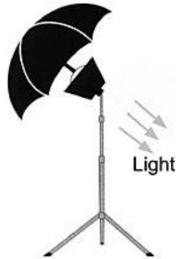
Figure 4: - Diagram of a reflective umbrella positioned with the concave side of the umbrella pointed at the subject and the flash is shone on the inside of the umbrella.
