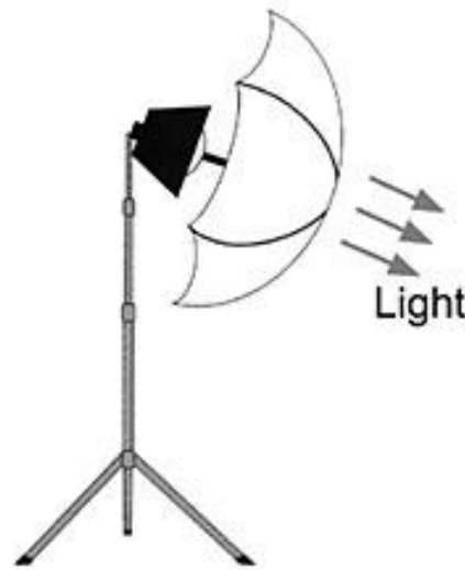
Figure 5: - Diagram of a white umbrella positioned with the convex side pointed at the subject and the flash is shone through the umbrella imitating a softbox effect.
